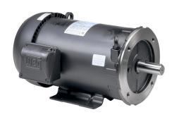
WEG Electric S premium efficiency AC induction motor, general purpose and inverter rated, 5hp, 3-phase, 208-230/460 VAC, 1800rpm, TEFC, 184TC frame, rolled steel, C-face/rigid base mount.
