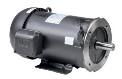
WEG Electric S premium efficiency AC induction motor, general purpose and inverter rated, 5hp, 3-phase, 208-230/460 VAC, 1800rpm, TEFC, NEMA 184TC frame, rolled steel, C-face/rigid base mount.
