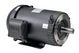
WEG Electric S premium efficiency AC induction motor, general purpose and inverter rated, 5hp, 3-phase, 208-230/460 VAC, 1200rpm, TEFC, NEMA 215TC frame, rolled steel, C-face/rigid base mount.
