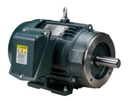
Toshiba SD premium efficiency AC induction motor, highperformance inverter duty and severe duty, 3hp, 3-phase, 230/460 VAC, 1200rpm, TEFC, NEMA 213TC frame, cast iron, Cface/rigid base mount.
