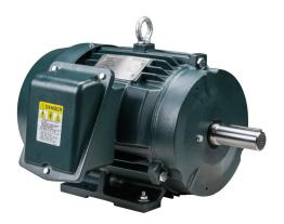
Toshiba SD premium efficiency AC induction motor, highperformance inverter duty and severe duty, 3hp, 3-phase, 230/460 VAC, 1200rpm, TEFC, NEMA 213T frame, cast iron, rigid base mount.
