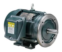
Toshiba SD premium efficiency AC induction motor, highperformance inverter duty and severe duty, 3hp, 3-phase, 230/460 VAC, 1800rpm, TEFC, NEMA 182TC frame, cast iron, Cface/rigid base mount.
