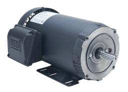
WEG Electric S premium efficiency AC induction motor, general purpose and inverter rated, 3hp, 3-phase, 208-230/460 VAC, 3600rpm, TEFC, NEMA 56HC frame, rolled steel, C-face/rigid base mount.
