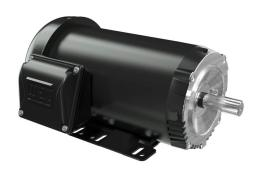
WEG Electric S premium efficiency AC induction motor, general purpose and inverter rated, 3hp, 3-phase, 208-230/460 VAC, 3600rpm, TEFC, NEMA 143/5TC frame, rolled steel, C-face/rigid base mount.
