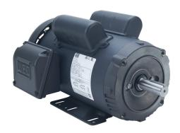
WEG Electric S standard efficiency AC induction motor, general purpose, 3hp, 1-phase, 208-230/460 VAC, 3600rpm, TEFC, NEMA 143/5TC frame, rolled steel, C-face/rigid base mount.
