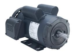
WEG Electric S standard efficiency AC induction motor, general purpose, 3hp, 1-phase, 208-230/460 VAC, 3600rpm, TEFC, 143/5TC frame, rolled steel, C-face/rigid base mount.
