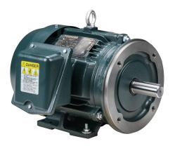
Toshiba SD premium efficiency AC induction motor, highperformance inverter duty and severe duty, 3hp, 3-phase, 230/460 VAC, 3600rpm, TEFC, NEMA 182TC frame, cast iron, Cface/rigid base mount.
