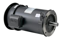
WEG Electric S premium efficiency AC induction motor, general purpose and inverter rated, 3hp, 3-phase, 208-230/460 VAC, 1800rpm, TEFC, NEMA 182TC frame, rolled steel, C-face mount. Drip cover included.
