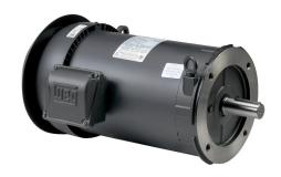
WEG Electric S premium efficiency AC induction motor, general purpose and inverter rated, 3hp, 3-phase, 208-230/460 VAC, 1800rpm, TEFC, 182TC frame, rolled steel, C-face mount. Drip cover included.
