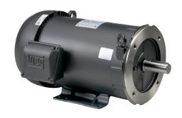
WEG Electric S premium efficiency AC induction motor, general purpose and inverter rated, 3hp, 3-phase, 208-230/460 VAC, 1800rpm, TEFC, NEMA 182TC frame, rolled steel, C-face/rigid base mount.
