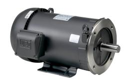
WEG Electric S premium efficiency AC induction motor, general purpose and inverter rated, 3hp, 3-phase, 208-230/460 VAC, 1800rpm, TEFC, 182TC frame, rolled steel, C-face/rigid base mount.
