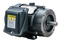
Toshiba SD premium efficiency AC induction motor, highperformance inverter duty and severe duty, 2hp, 3-phase, 230/460 VAC, 1800rpm, TEFC, NEMA 145TC frame, cast iron, Cface/rigid base mount.
