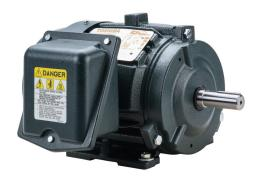
Toshiba SD premium efficiency AC induction motor, high-performance inverter duty and severe duty, 2hp, 3-phase, 230/460 VAC, 1800rpm, TEFC, 145T frame, cast iron, rigid base mount.
