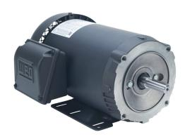
WEG Electric S premium efficiency AC induction motor, general purpose and inverter rated, 2hp, 3-phase, 208-230/460 VAC, 3600rpm, TEFC, NEMA 56HC frame, rolled steel, C-face/rigid base mount.
