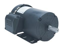
WEG Electric S premium efficiency AC induction motor, general purpose and inverter rated, 2hp, 3-phase, 208-230/460 VAC, 3600rpm, TEFC, 143/5 frame, rolled steel, rigid base mount.
