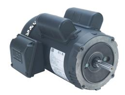
WEG Electric S standard efficiency AC induction motor, general purpose, 2hp, 1-phase, 115/208-230 VAC, 3600rpm, TEFC, NEMA 56C frame, rolled steel, C-face mount.
