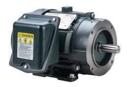
Toshiba SD premium efficiency AC induction motor, high-performance inverter duty and severe duty, 2hp, 3-phase, 230/460 VAC, 3600rpm, TEFC, 145TC frame, cast iron, C-face/rigid base mount.
