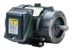
Toshiba SD premium efficiency AC induction motor, highperformance inverter duty and severe duty, 2hp, 3-phase, 230/460 VAC, 3600rpm, TEFC, NEMA 145TC frame, cast iron, Cface/rigid base mount.
