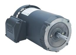
WEG Electric S premium efficiency AC induction motor, general purpose and inverter rated, 2hp, 3-phase, 208-230/460 VAC, 1800rpm, TEFC, NEMA 56C frame, rolled steel, C-face mount.
