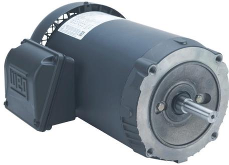
WEG Electric S premium efficiency AC induction motor, general purpose and inverter rated, 2hp, 3-phase, 208-230/460 VAC, 1800rpm, TEFC, NEMA 56C frame, rolled steel, C-face mount.
