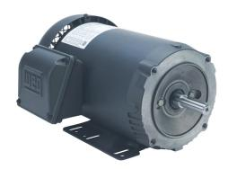
WEG Electric S premium efficiency AC induction motor, general purpose and inverter rated, 2hp, 3-phase, 208-230/460 VAC, 1800rpm, TEFC, 56HC frame, rolled steel, C-face/rigid base mount.
