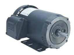
WEG Electric S premium efficiency AC induction motor, general purpose and inverter rated, 2hp, 3-phase, 208-230/460 VAC, 1800rpm, TEFC, NEMA 56HC frame, rolled steel, C-face/rigid base mount.
