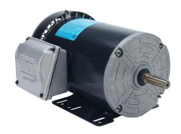
WEG Electric S premium efficiency AC induction motor, general purpose and inverter rated, 2hp, 3-phase, 208-230/460 VAC, 1800rpm, TEFC, NEMA 56H frame, rolled steel, rigid base mount.
