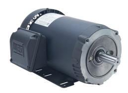
WEG Electric S premium efficiency AC induction motor, general purpose and inverter rated, 2hp, 3-phase, 208-230/460 VAC, 1800rpm, TEFC, NEMA 143/5TC frame, rolled steel, C-face/rigid base mount.
