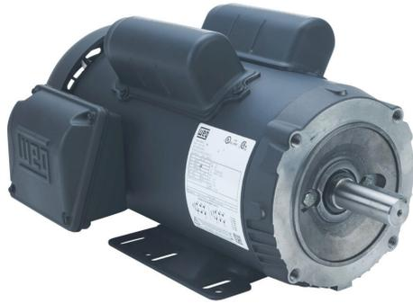
WEG Electric S standard efficiency AC induction motor, general purpose, 2hp, 1-phase, 115/208-230 VAC, 1800rpm, TEFC, 143/5TC frame, rolled steel, C-face/rigid base mount.
