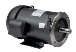
WEG Electric S premium efficiency AC induction motor, general purpose and inverter rated, 2hp, 3-phase, 208-230/460 VAC, 1200rpm, TEFC, NEMA 184TC frame, rolled steel, C-face/rigid base mount.
