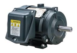
Toshiba SD premium efficiency AC induction motor, high-performance inverter duty and severe duty, 1hp, 3-phase, 230/460 VAC, 1200rpm, TEFC, NEMA 145T frame, cast iron, rigid base mount.
