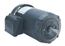
WEG Electric S premium efficiency AC induction motor, general purpose and inverter rated, 1-1/2hp, 3-phase, 208-230/460 VAC, 1800rpm, TEFC, NEMA 56C frame, rolled steel, C-face mount.
