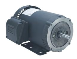
WEG Electric S premium efficiency AC induction motor, general purpose and inverter rated, 1-1/2hp, 3-phase, 208-230/460 VAC, 1800rpm, TEFC, NEMA 56HC frame, rolled steel, C-face/rigid base mount.
