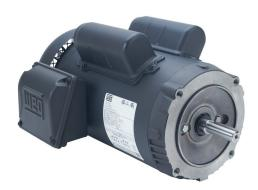
WEG Electric S standard efficiency AC induction motor, general purpose, 1-1/2hp, 1-phase, 115/208-230 VAC, 1800rpm, TEFC, NEMA 56C frame, rolled steel, C-face mount.
