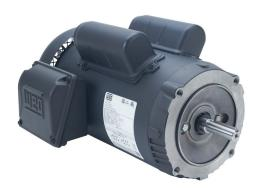
WEG Electric S standard efficiency AC induction motor, general purpose, 1-1/2hp, 1-phase, 115/208-230 VAC, 1800rpm, TEFC, 56C frame, rolled steel, C-face mount.
