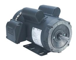
WEG Electric S standard efficiency AC induction motor, general purpose, 1-1/2hp, 1-phase, 115/208-230 VAC, 1800rpm, TEFC, NEMA 56HC frame, rolled steel, C-face/rigid base mount.
