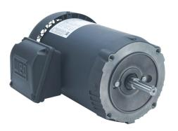
WEG Electric S premium efficiency AC induction motor, general purpose and inverter rated, 1-1/2hp, 3-phase, 208-230/460 VAC, 3600rpm, TEFC, 56C frame, rolled steel, C-face mount.
