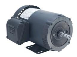
WEG Electric S premium efficiency AC induction motor, general purpose and inverter rated, 1-1/2hp, 3-phase, 208-230/460 VAC, 3600rpm, TEFC, NEMA 56C frame, rolled steel, C-face/rigid base mount.
