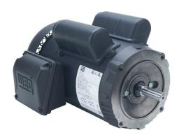
WEG Electric S standard efficiency AC induction motor, general purpose, 1-1/2hp, 1-phase, 115/208-230 VAC, 3600rpm, TEFC, NEMA 56C frame, rolled steel, C-face mount.
