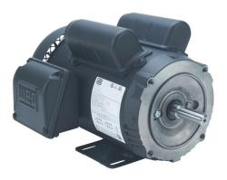
WEG Electric S standard efficiency AC induction motor, general purpose, 1-1/2hp, 1-phase, 115/208-230 VAC, 3600rpm, TEFC, NEMA 56C frame, rolled steel, C-face/rigid base mount.
