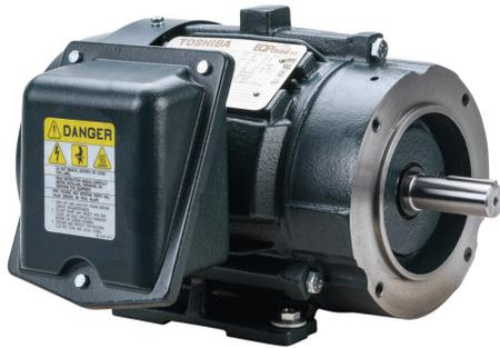
Toshiba SD premium efficiency AC induction motor, high-performance inverter duty and severe duty, 1hp, 3-phase, 230/460 VAC, 1800rpm, TEFC, NEMA 143TC frame, cast iron, C-face/rigid base mount.
