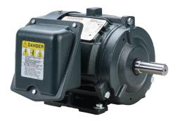
Toshiba SD premium efficiency AC induction motor, highperformance inverter duty and severe duty, 1hp, 3-phase, 230/460 VAC, 1800rpm, TEFC, NEMA 143T frame, cast iron, rigid base mount.
