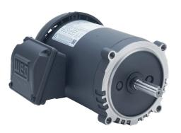
WEG Electric S premium efficiency AC induction motor, general purpose and inverter rated, 1hp, 3-phase, 208-230/460 VAC, 3600rpm, TEFC, NEMA 56C frame, rolled steel, C-face mount.
