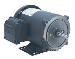
WEG Electric S premium efficiency AC induction motor, general purpose and inverter rated, 1hp, 3-phase, 208-230/460 VAC, 3600rpm, TEFC, NEMA 56C frame, rolled steel, C-face/rigid base mount.
