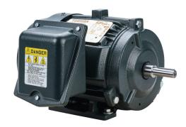
Toshiba SD premium efficiency AC induction motor, highperformance inverter duty and severe duty, 1hp, 3-phase, 230/460 VAC, 3600rpm, TEFC, NEMA 56 frame, cast iron, rigid base mount.
