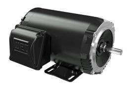
WEG Electric S premium efficiency AC induction motor, high-performance inverter duty, 1hp, 3-phase, 230/460 VAC, 1800rpm, TENV, 56CZ frame, rolled steel, C-face/rigid base mount.
