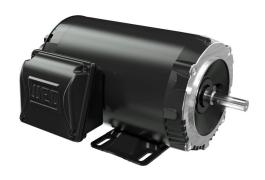
WEG Electric S premium efficiency AC induction motor, highperformance inverter duty, 1hp, 3-phase, 230/460 VAC, 1800rpm, TENV, NEMA 56CZ frame, rolled steel, C-face/rigid base mount.
