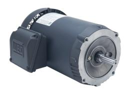
WEG Electric S premium efficiency AC induction motor, general purpose and inverter rated, 1hp, 3-phase, 208-230/460 VAC, 1800rpm, TEFC, NEMA 56C frame, rolled steel, C-face mount.
