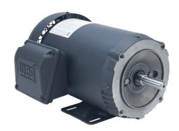
WEG Electric S premium efficiency AC induction motor, general purpose and inverter rated, 1hp, 3-phase, 208-230/460 VAC, 1800rpm, TEFC, NEMA 56C frame, rolled steel, C-face/rigid base mount.
