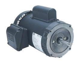
WEG Electric S standard efficiency AC induction motor, general purpose, 1hp, 1-phase, 115/208-230 VAC, 1800rpm, TEFC, NEMA 56C frame, rolled steel, C-face mount.
