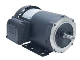
WEG Electric S premium efficiency AC induction motor, general purpose and inverter rated, 1hp, 3-phase, 208-230/460 VAC, 1200rpm, TEFC, NEMA 56HC frame, rolled steel, C-face/rigid base mount.
