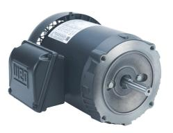
WEG Electric S standard efficiency AC induction motor, general purpose and inverter rated, 3/4hp, 3-phase, 208-230/460 VAC, 3600rpm, TEFC, NEMA 56C frame, rolled steel, C-face mount.
