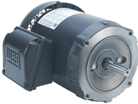
WEG Electric S standard efficiency AC induction motor, general purpose and inverter rated, 3/4hp, 3-phase, 208-230/460 VAC, 3600rpm, TEFC, NEMA 56C frame, rolled steel, C-face mount.
