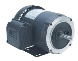
WEG Electric S standard efficiency AC induction motor, general purpose and inverter rated, 3/4hp, 3-phase, 208-230/460 VAC, 3600rpm, TEFC, NEMA 56C frame, rolled steel, C-face/rigid base mount.
