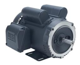
WEG Electric S standard efficiency AC induction motor, general purpose, 3/4hp, 1-phase, 115/208-230 VAC, 3600rpm, TEFC, 56C frame, rolled steel, C-face/rigid base mount.
