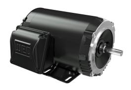
WEG Electric S premium efficiency AC induction motor, highperformance inverter duty, 3/4hp, 3-phase, 230/460 VAC, 1800rpm, TENV, NEMA 56CZ frame, rolled steel, C-face/rigid base mount.
