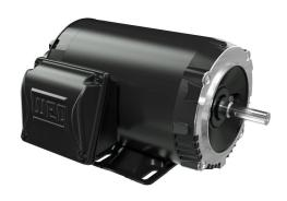
WEG Electric S premium efficiency AC induction motor, highperformance inverter duty, 3/4hp, 3-phase, 230/460 VAC, 1800rpm, TENV, 56CZ frame, rolled steel, C-face/rigid base mount.
