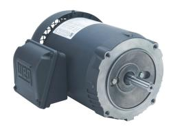
WEG Electric S standard efficiency AC induction motor, general purpose and inverter rated, 3/4hp, 3-phase, 208-230/460 VAC, 1800rpm, TEFC, NEMA 56C frame, rolled steel, C-face mount.
