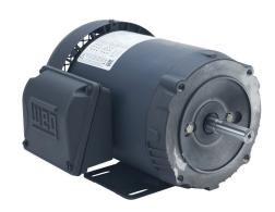
WEG Electric S standard efficiency AC induction motor, general purpose and inverter rated, 3/4hp, 3-phase, 208-230/460 VAC, 1800rpm, TEFC, 56C frame, rolled steel, C-face/rigid base mount.
