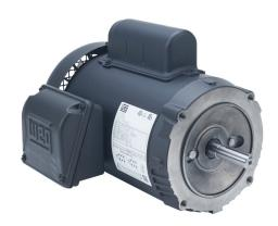
WEG Electric S standard efficiency AC induction motor, general purpose, 3/4hp, 1-phase, 115/208-230 VAC, 1800rpm, TEFC, 56C frame, rolled steel, C-face mount.
