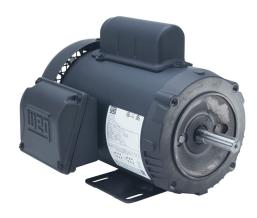
WEG Electric S standard efficiency AC induction motor, general purpose, 3/4hp, 1-phase, 115/208-230 VAC, 1800rpm, TEFC, 56C frame, rolled steel, C-face/rigid base mount.
